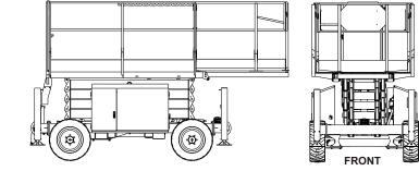
Danger: Standard models described in this brochure are NON-INSULATED and do not provide electrocution protection from contact with or close proximity to energised conductors which is pointed out on the decals and placards attached to the machine.
